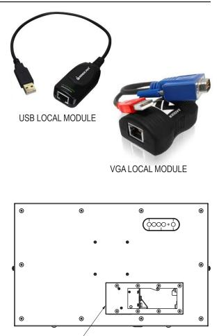
KVM REMOTE MODULE (COVER PLATE NOT SHOWN FOR CLARITY)
